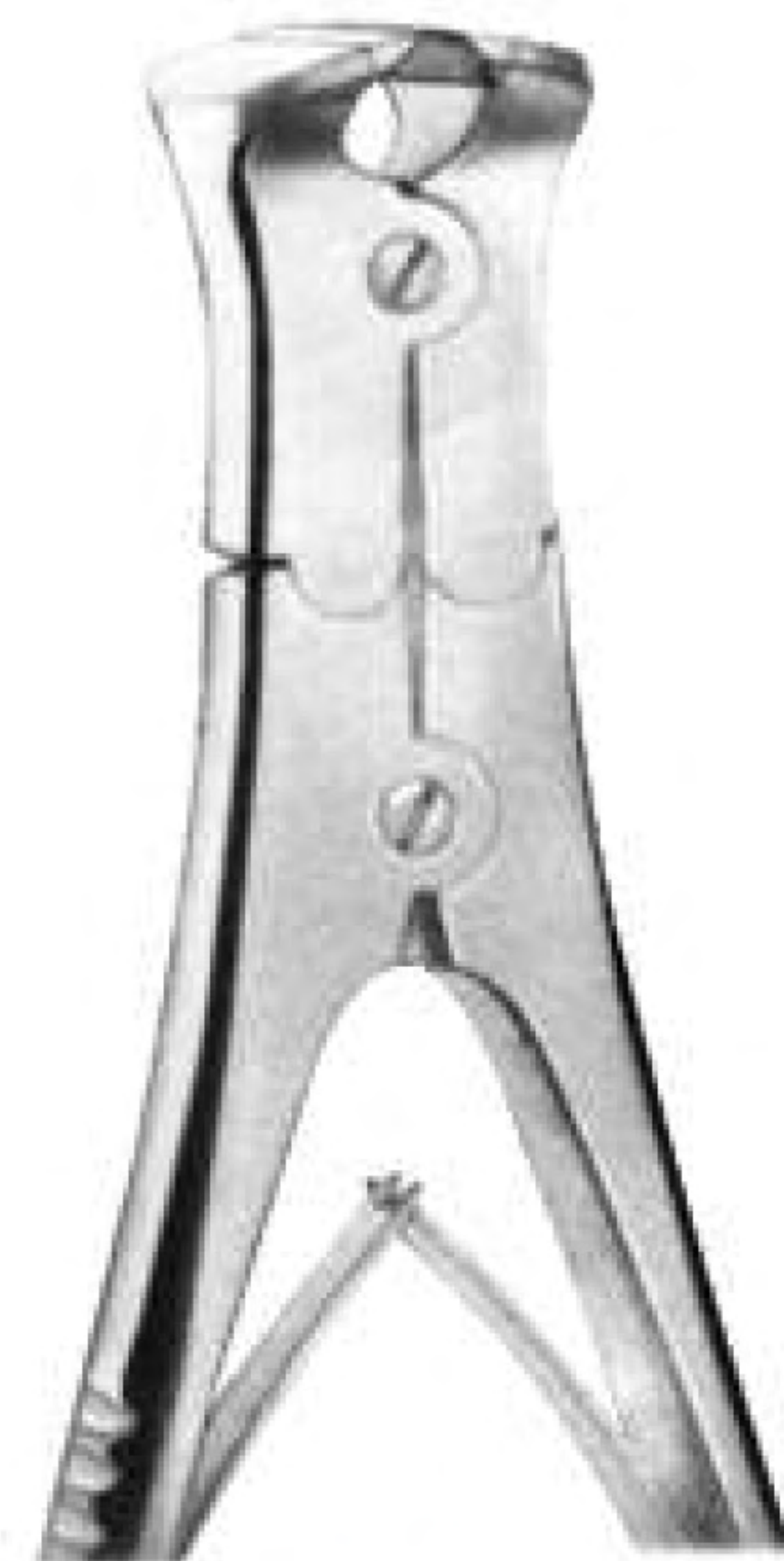
2419 Wire cutter. For ligature wires and pins. It is strong enough to bend archwire ends after distal cutting. Maximum cutting capacity: wires up to 1,5 mm. (.044"). With tungsten carbide insert.
